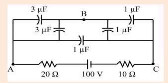
**Q7.** Find the potential difference Va - Vb in the circuits shown in figures given below.
